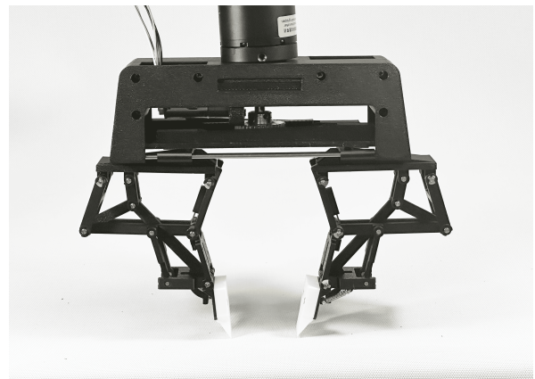
Fig. 1. The SPARK Hand, a robotic end-effector consisting of two SPARK fingers on a single base, capable of performing both parallel pinching and scooping grasps.
